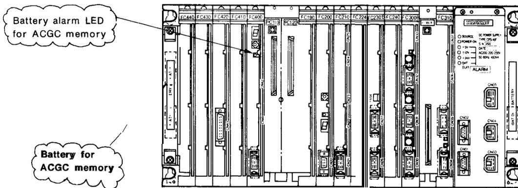
Fig. 2.4 Battery Layout (14" ACGC NC Rack 1)
