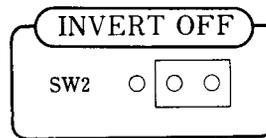
**Note** This switch activates or deactivates the function for using logical "1" as the logic when contact is closed, regardless of +24 V/0<sub>24</sub>.
