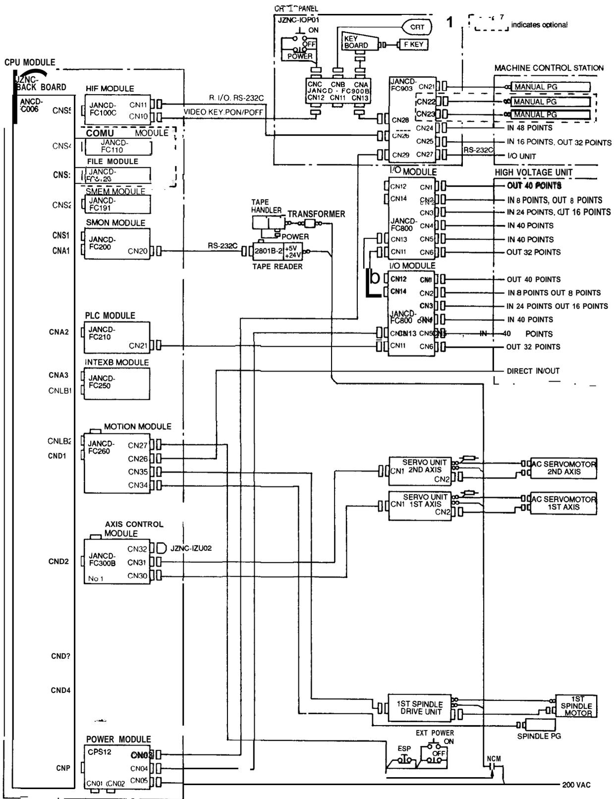
Fig. 1.8 Interconnection Diagram [Y AS NAC-i80LB for Lathe]
