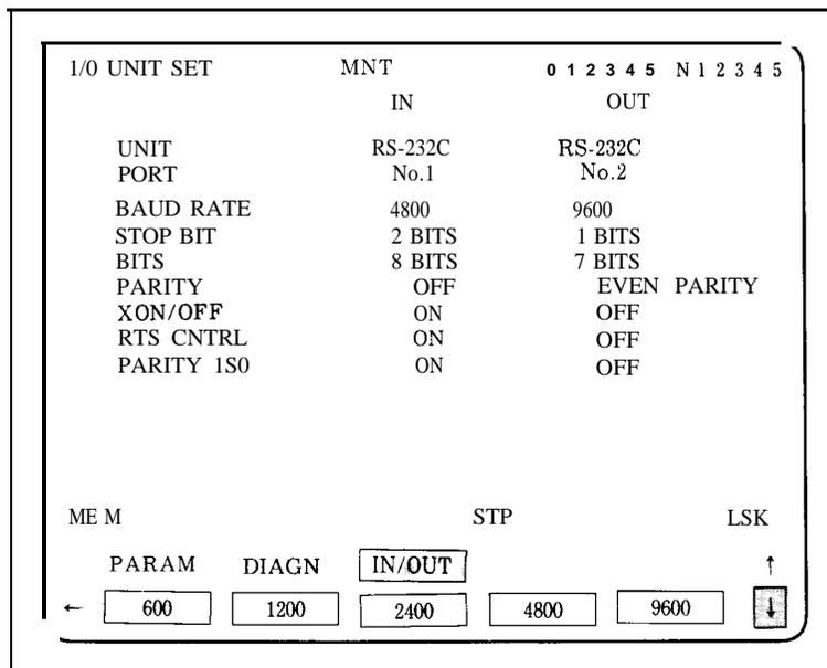
Fig. 4.7 Setting of Serial Interface
