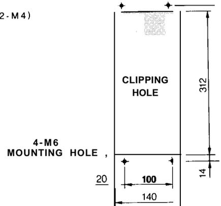
Mounting Hole Processing Diagram
