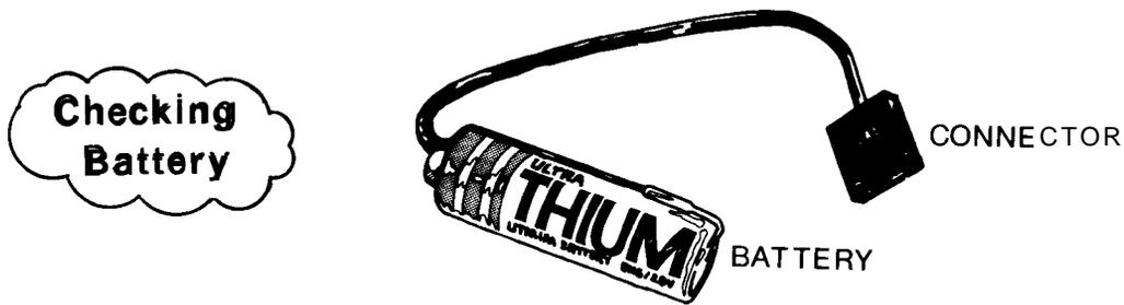
Make sure that "BAT" is not displayed on the lower right portion of the CRT screen at power ON. If it is displayed, the battery must be replaced within a month.
