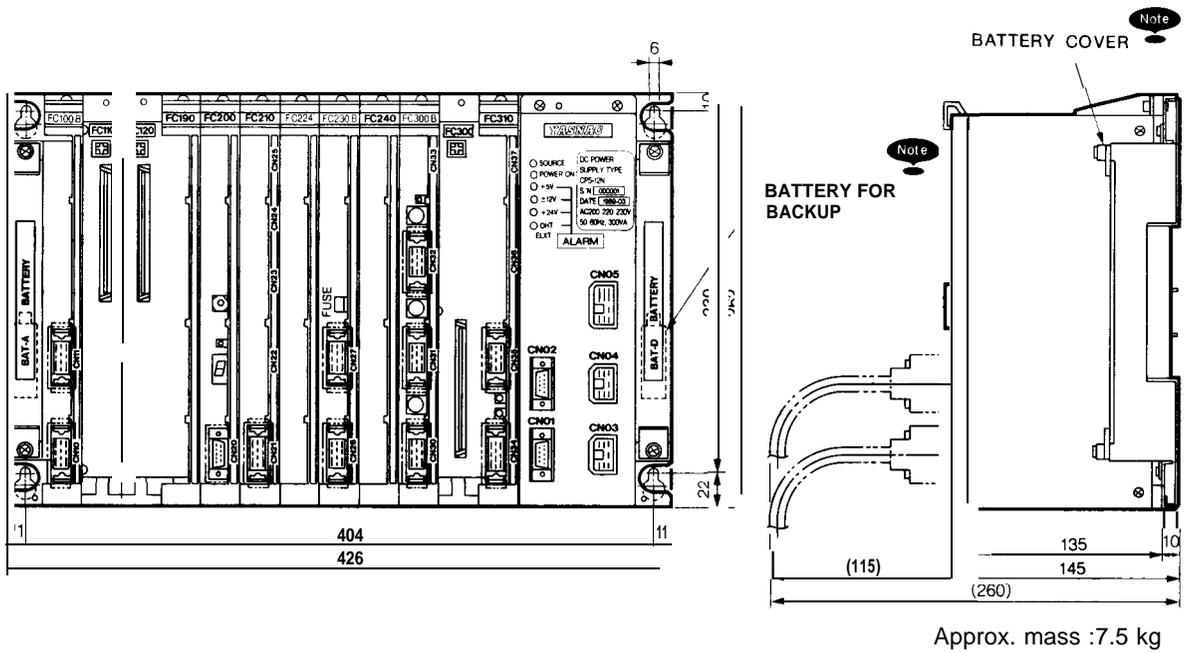
**Note** When replacing the battery for backup, remove the battery cover. (one at each side)
