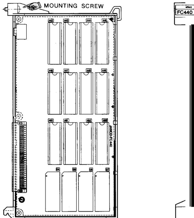
This module contains CMOS RAM in which ACGC application programs are stored. Accordingly, their contents must be copied when replacing the module,
