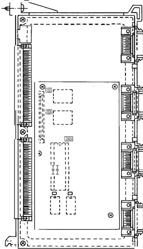
**This figure shows model JANCD-FC265 attached to model JANCD-FC260.**
