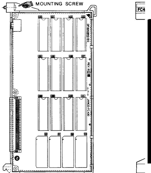
This module contains CMOS RAM in which **ACGC** application programs are stored. Accordingly, their contents must be copied when replacing the module.
