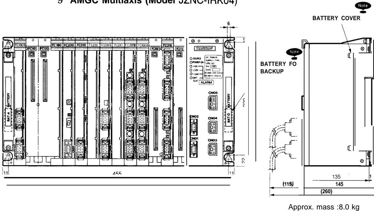
**Note** When replacing the battery for backup, remove the battery cover. (one at each side)
