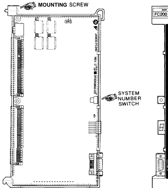
This module contains CMOS RAM in which NC program parameter values and offset values are stored. Accordingly, their contents must be copied when replacing the module.
