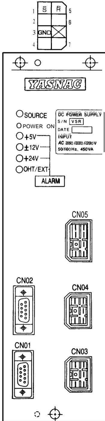
Fig. 4.9 External View of Power Supply Unit
